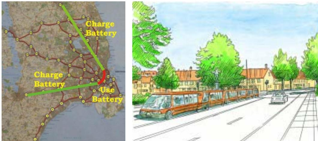
A RUF “tram” solution is much more attractive. It consists of a “train” of maxi-rufs and/or midi-rufs coupled together to form a “tram”. No rails are needed because it runs on rubber wheels. No overhead wires are needed because it runs on battery power. This is possible because the vehicles makes use of the rail network in order to recharge the batteries in between the tram trips.
